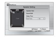
Use the Test Tone feature to check the speaker connections.
